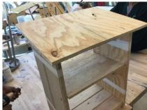
Step 5: Connect back to sides and roof
