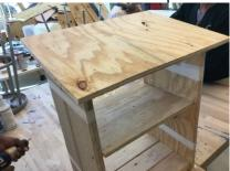
Using the 1/8" Drill Bit, drill a four medium sized screws into each corner of the roof
